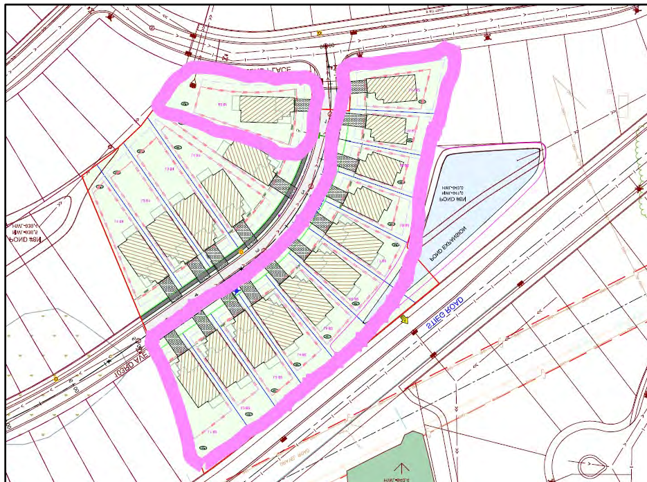
Figure 1: Lots highlighted in pink must provide architectural upgrades on elevations that face a public right-of-way or park.
