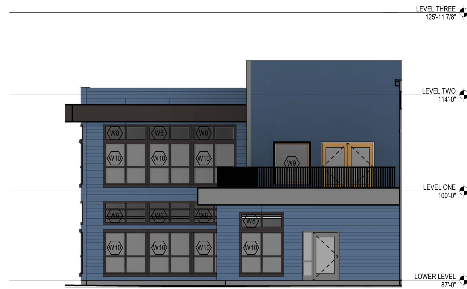
10 A3.3 AREA C - TOWN CENTER SOUTHEAST ELEVATION 1/8" = 1'-0"
